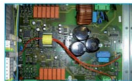
Main power board for rectification and inversion
