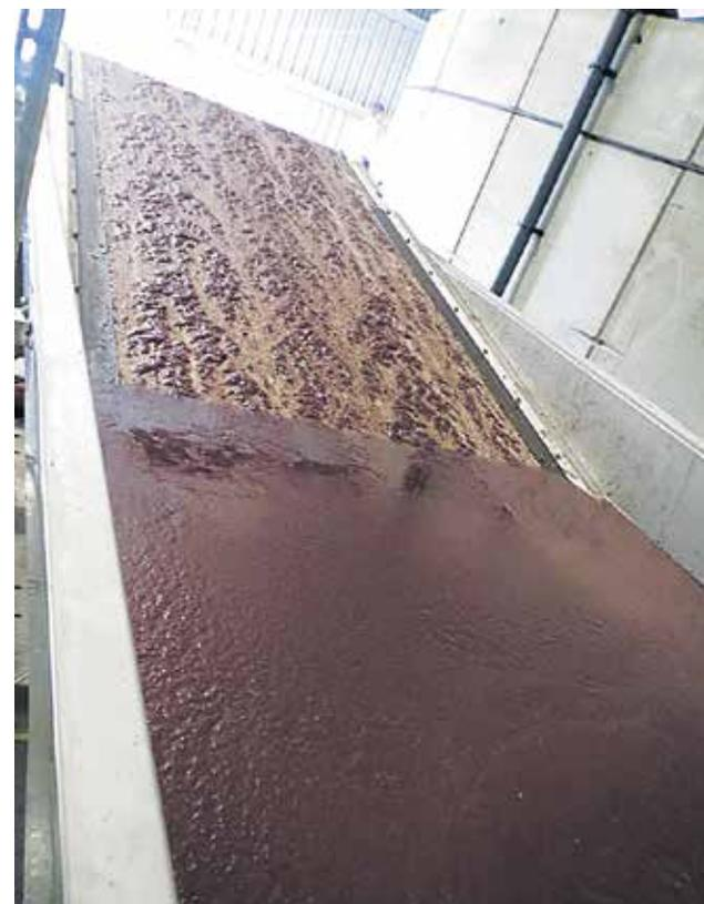
Belt separator removing flocculated sludge. It becomes a valuable by-product of the hatchery process.
